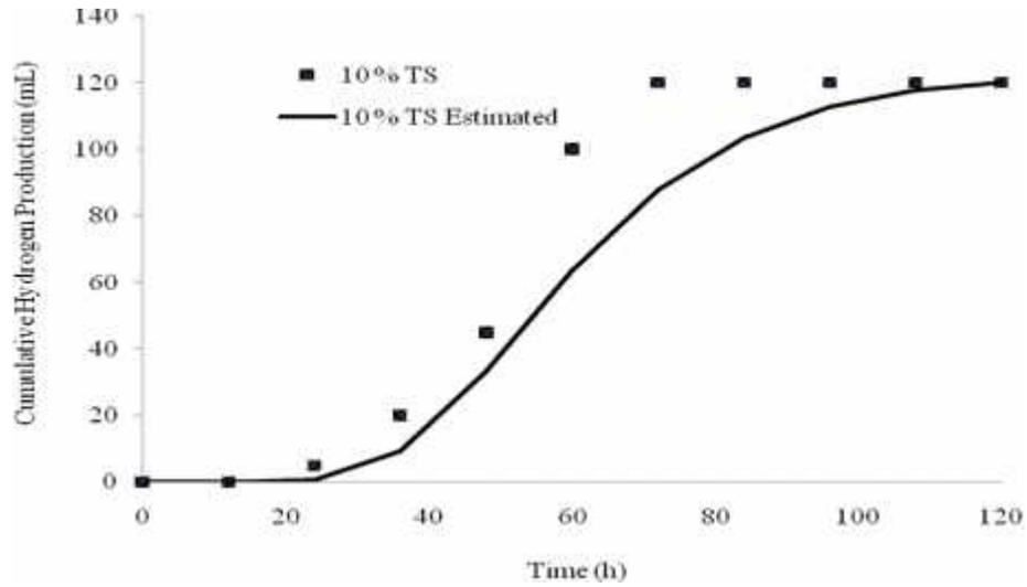
Figure 3. Cumulative Hydrogen production at 55 °C
