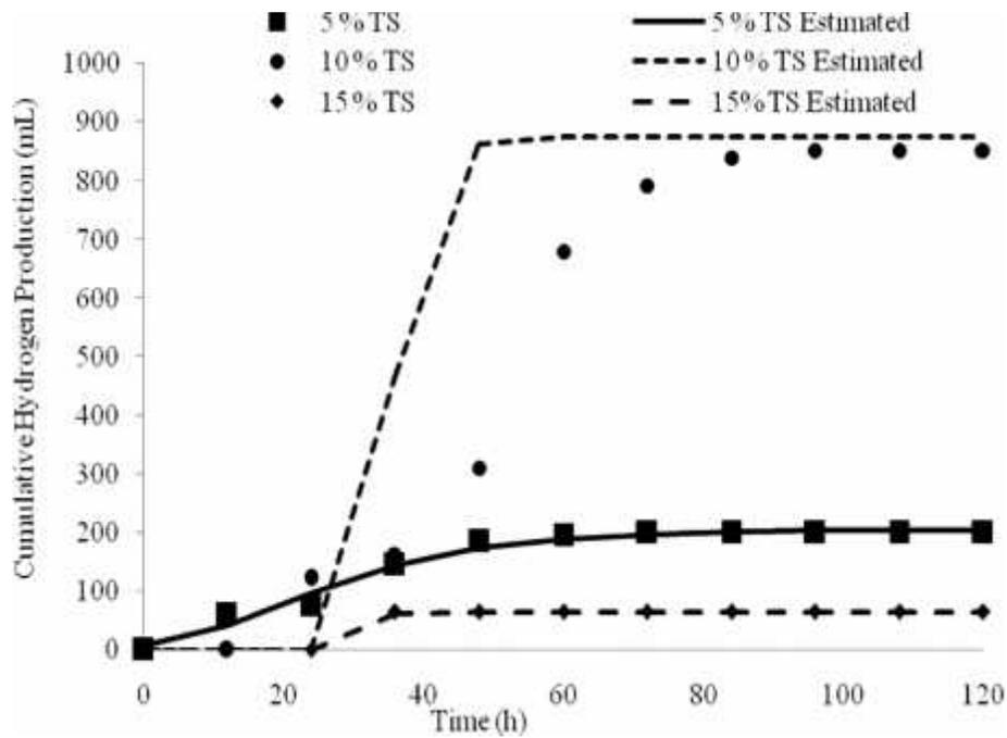
Figure 2. Cumulative hydrogen production at 37 °C
