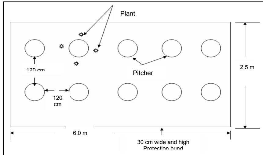
Figure 2.A layout showing a pitcher irrigation method
