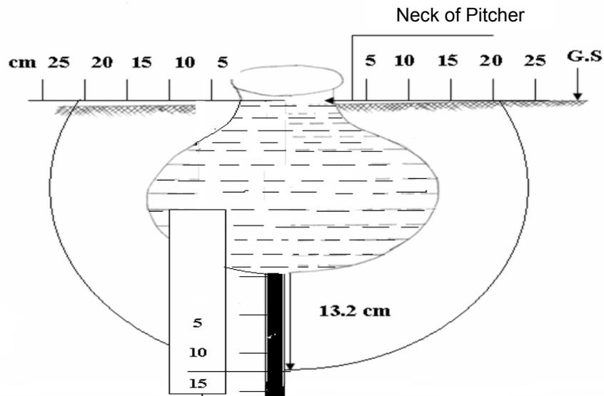
Figure 5. Schematic diagram of the wetting front of Pitcher
