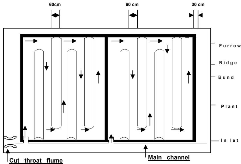
Figure 4. Layout plan of furrow irrigation method
